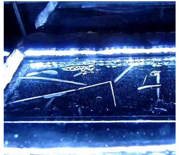
Fantastic double decay from a thorium based mineral. Right : thoron gas introduced in the chamber
