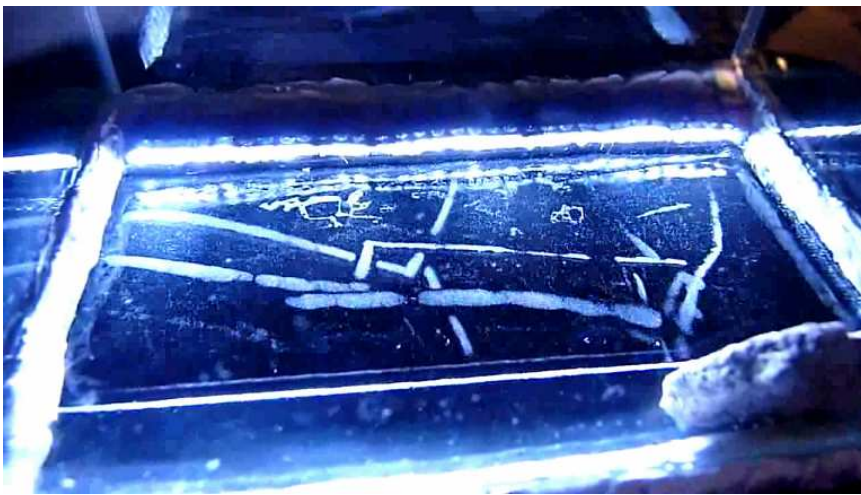
Fantastic double decay from a thorium based mineral. Right : thoron gas introduced in the chamber
