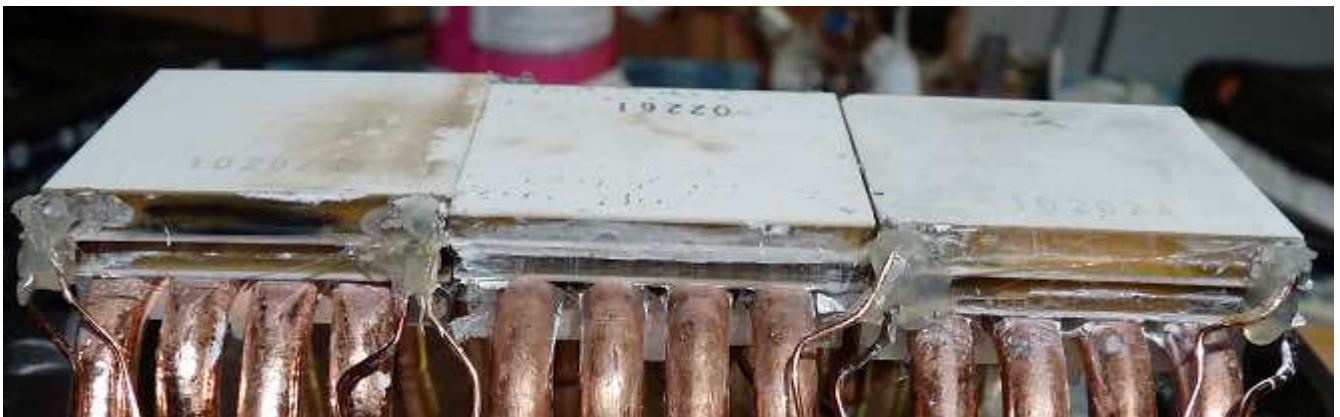
Good configuration of spacing, continuous surface of peltiers
