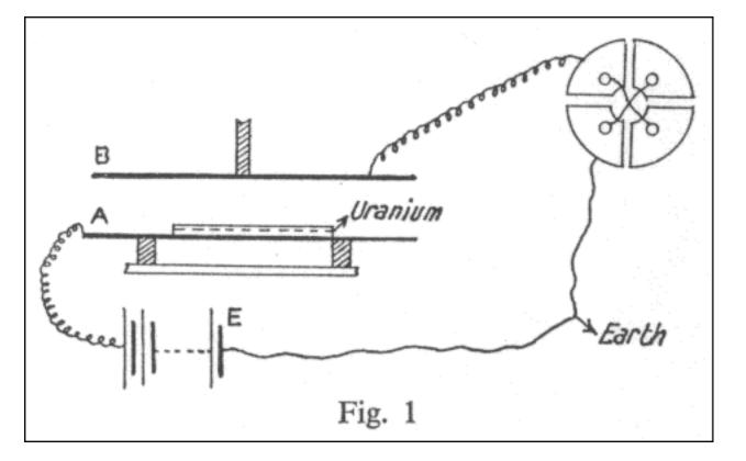
A uniform layer of powered uranium compound was spread on plate A and the rays allowed to ionize the gas between plates A and B. The amount of ionization is measured by the "saturation current" received at B when the potential difference between A and B is great enough to pull all the ions to the plates before they are able to recombine.
