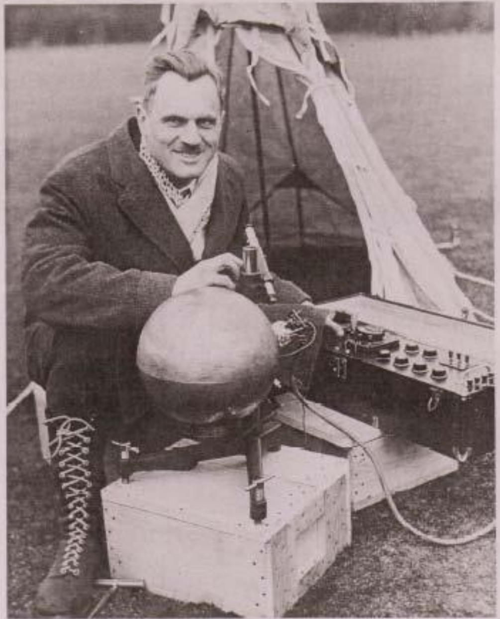
Fig. 6. Compton with the special ionization chamber which he designed and used for his world-wide cosmic-ray survey during 1931-33, which proved that cosmic rays are charged particles.
