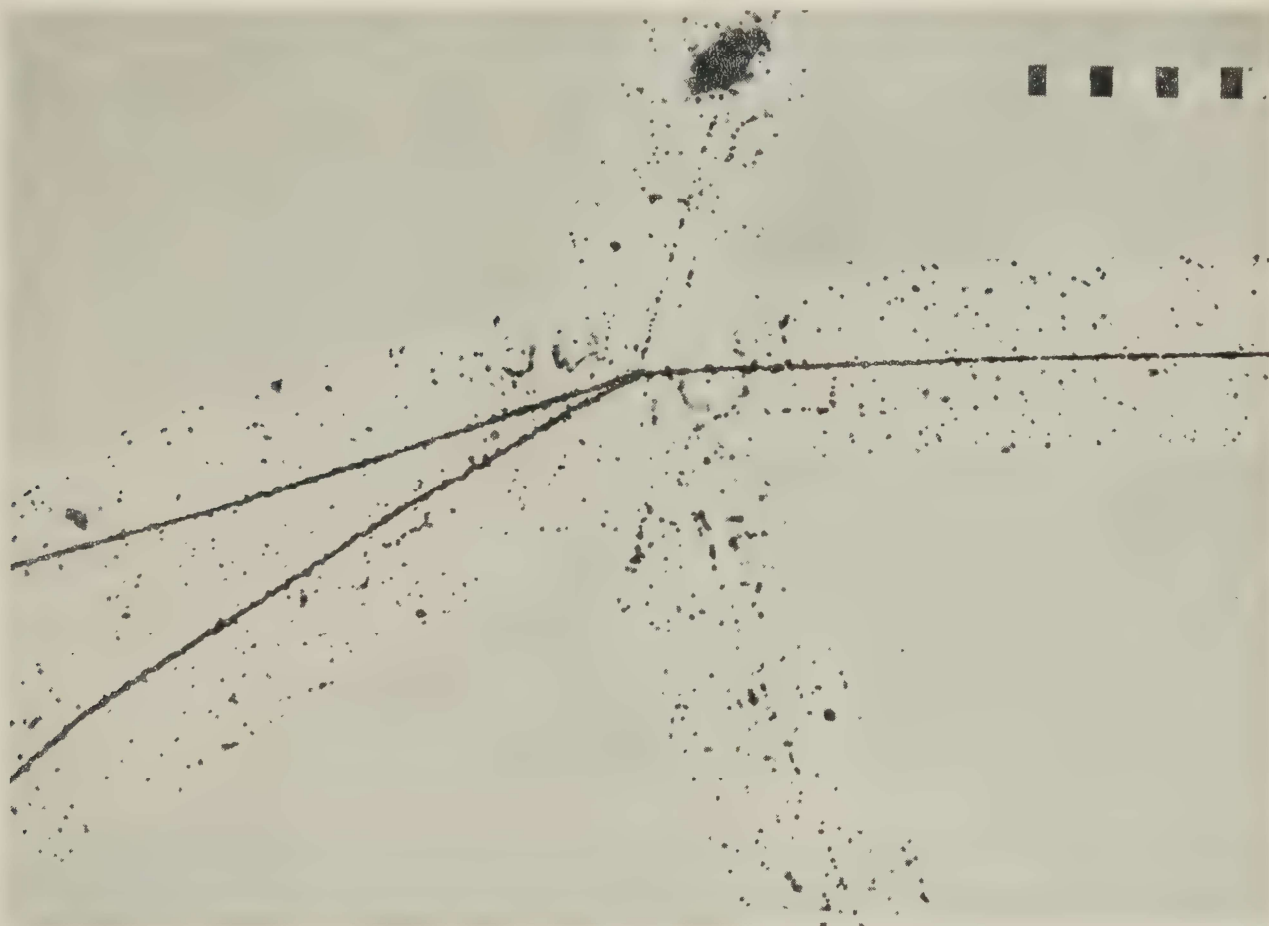
Figure 5. A disintegration produced by a fast charged particle at a depth of 20 m. water. The angle of deviation of the fast particle is 30^\circ , the largest that has so far been observed in underground stars of this type. Observer: E. P. GEORGE.
